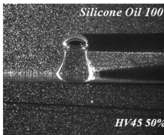
Figure 6. Example of images obtained at the interface with tracer particles (reflection comes from the interface).
